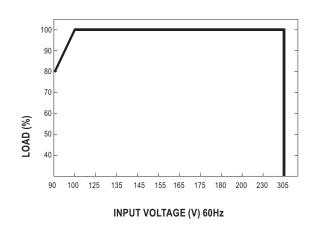
$\ensuremath{\aleph}$  De-rating is needed under low input voltage.
