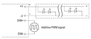
"DO NOT connect "DIM- to -V"
