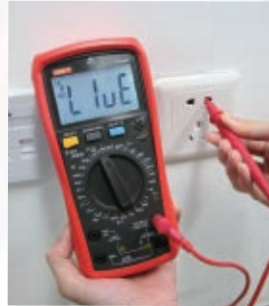
Live and nature wires identification
