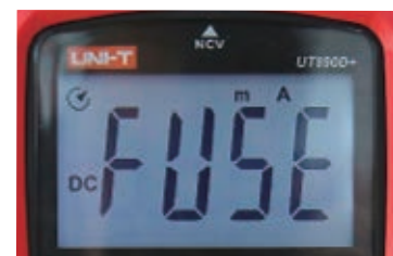
Fuse blowing alarm (mA only)
